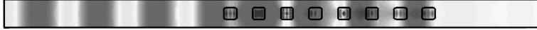
FIG. 3.1. Pressure in the sonic crystal for a long wavelength plane wave incident from the left.
