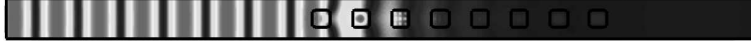
FIG. 3.3. Snapshot of RMS pressure distribution in space in the sonic crystal for a plane wave incident from the left.
